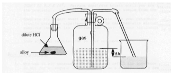
2. A demonstration apparatus should also be displayed on your instructor's bench. The generator flask is a 250 mL Erlenmeyer flask fitted with a one-hole stopper; the beaker is a 1000 mL beaker. Insert the glass tubes in the two-hole stopper of the large bottle with equal treatment and care. The generator flask should be placed in a beaker.
